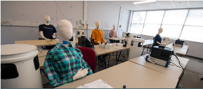
Retrofit package validation in LBNL's FLEXLAB. Occupant emulators and programmable plug loads are shown at desks in a classroom configuration.
